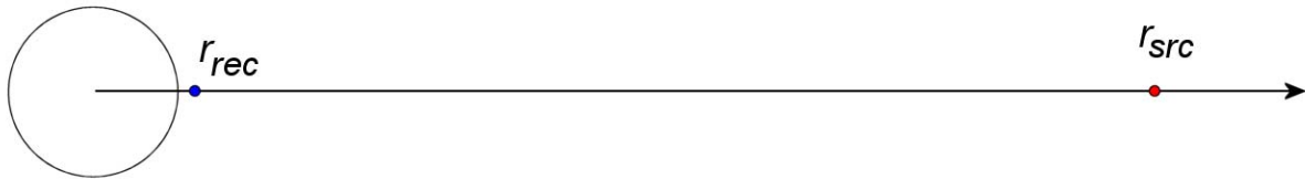
Figure 1. Set-up for the calculations. A rigid sphere of radius a scatters the incoming field from the monopole placed at r_{src} . The sound pressure is evaluated at r_{rec} .
